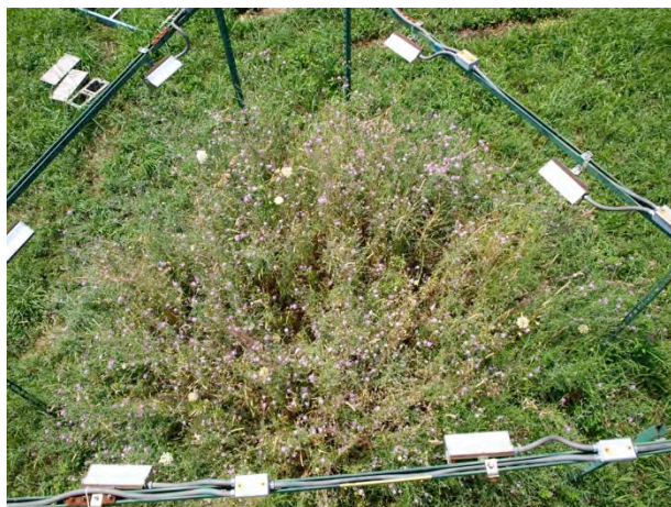
One of the heated plots shown from above. The silver boxes are electric heaters that raised the temperature inside the ring.
